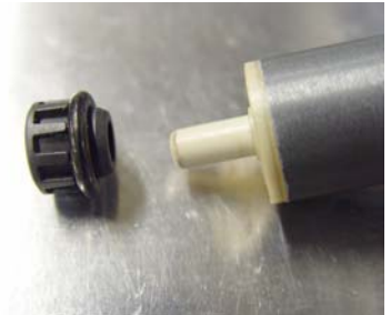
The bearing after removal from the shaft.
